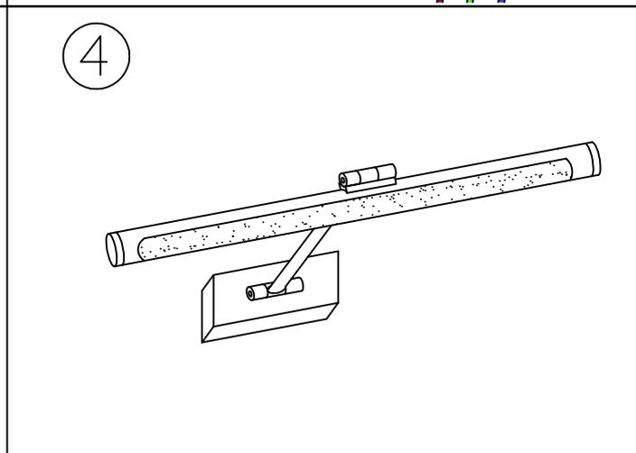
EN: Don't pull the arm without releasing the screws , this may lead the gear to disfunction.
